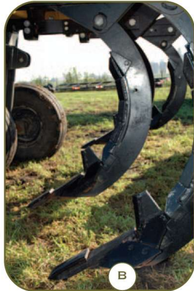
SUBSOILER SHANKS: (A) STRAIGHT, (B) PARABOLIC, AND (C) BENT LEG.
